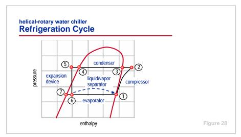
The theoretical vapor-compression refrigeration cycle for a helical-rotary water chiller can be plotted on a pressure-enthalpy chart.
